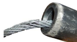
Wire breakage on the black grip sleeve
