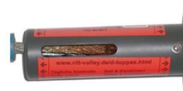
Rust at the cable in the grip sleeve
