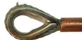
Wire breakage at the thimble
