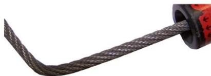
Remaining cable deformation
