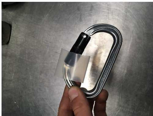
Put on the shrinking tube
